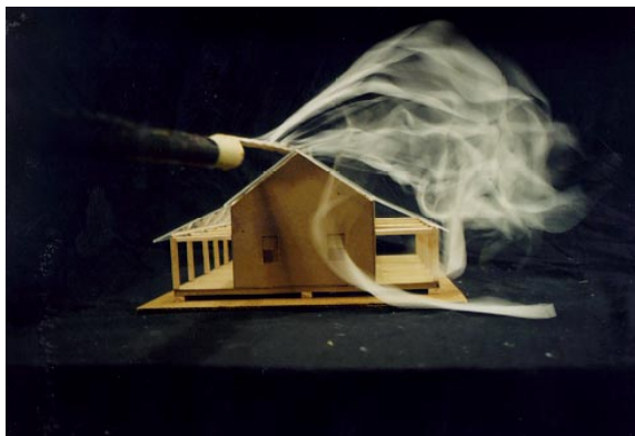
Turbulences are created on the leeward (north) side of the roof.
