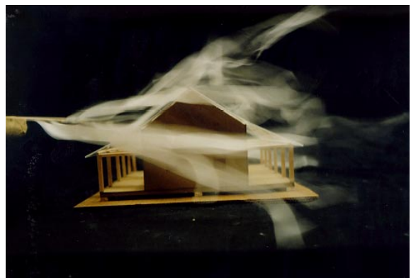
The image above shows most air travels up and over the roof while some continues level and moves around the house.
