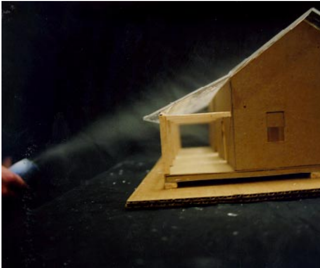
image demonstrating smoke test technique.
