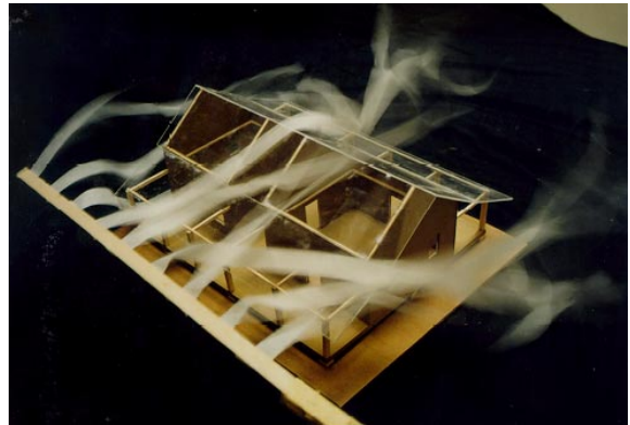
The image above shows air above ground mainly flows above and on the east or west side of the dogtrot. A smaller volume of air travels through the breezeway but at a greater velocity.
