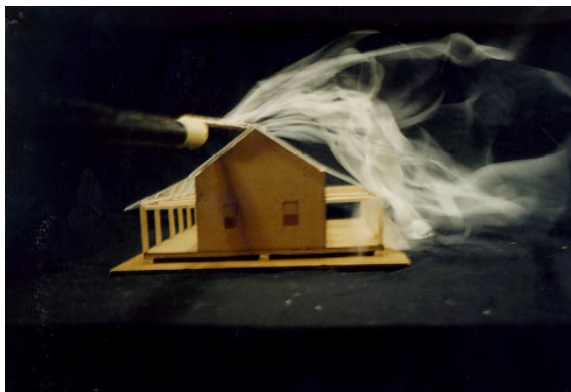
Air is directed over the roof, creating turbulence and then it is directed down after it passes over the roof.
